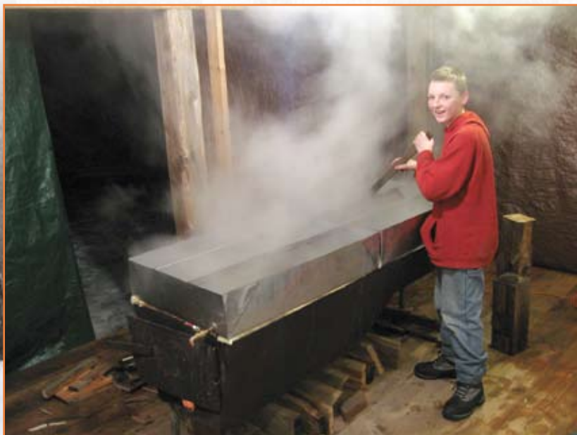
Tim in the sugar shack he and DJ constructed, stirring sap in the evaporator pan Grampa built. The pans sit on an oven called an arch. This year Grampa even built a new arch.
